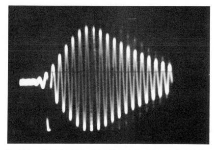
FIG. 1 (a). — Pulse signal seen on receiver c.r.t. at short range from station, showing gate pulse (referred to later) on third cycle.
