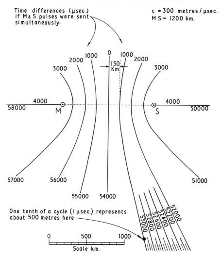
FIG. 4. — Typical Loran C pattern numbering (microseconds).
