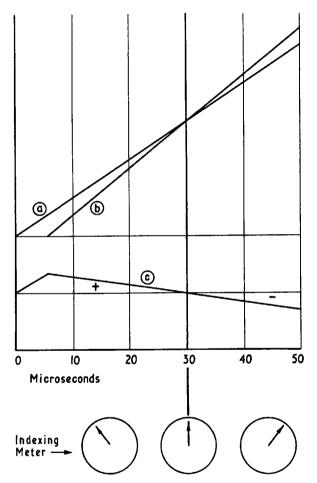
FIG. 6. -- Generation of indexing control signal from received pulse. Waveform (a), representing start of received pulse, is delayed and amplified to produce waveform (b) such that the two reach equal amplitude at the required 30 microsecond point. Subtracting (b) from (a) results in the control signal (c), which operates the meter as shown.
