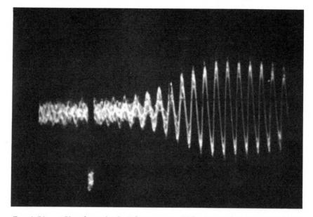
Fig. 1 (b). — Signal received at long range, with strong skywave component arriving after gate pulse.
