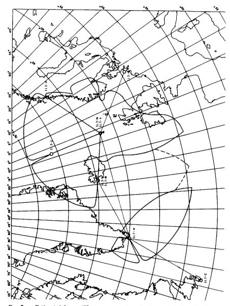
FIG. 7. — Estimated 5 n.m. (95 per cent) contour for Loran C in N. Atlantic area. This contour is based mainly on flight tests in the area. A maximum over-sea range of 1 000 n.m. per station is assumed, together with the presence of a 10-microsecond error due to fourth-cycle indexing. Station deployment is as predicted for March 1966. The dotted contour shows the coverage from Greenland-Iceland-Faroes, if this combination is retained.
