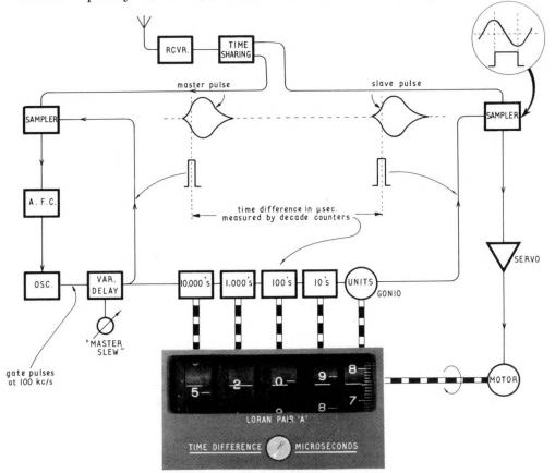
FIG. 5. - Loran C receiver AN/SPN-31 : method of deriving position line.
