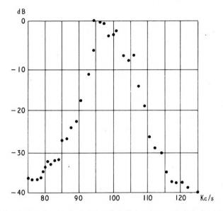
FIG. 3. — Approximate envelope of radiated spectrum at Sylt Loran C station.
