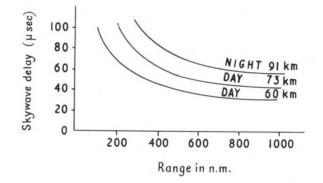
FIG. 2. — Average delay of single-hop skywave for three ionosphere heights (60 km height applies only to high northern latitudes).
